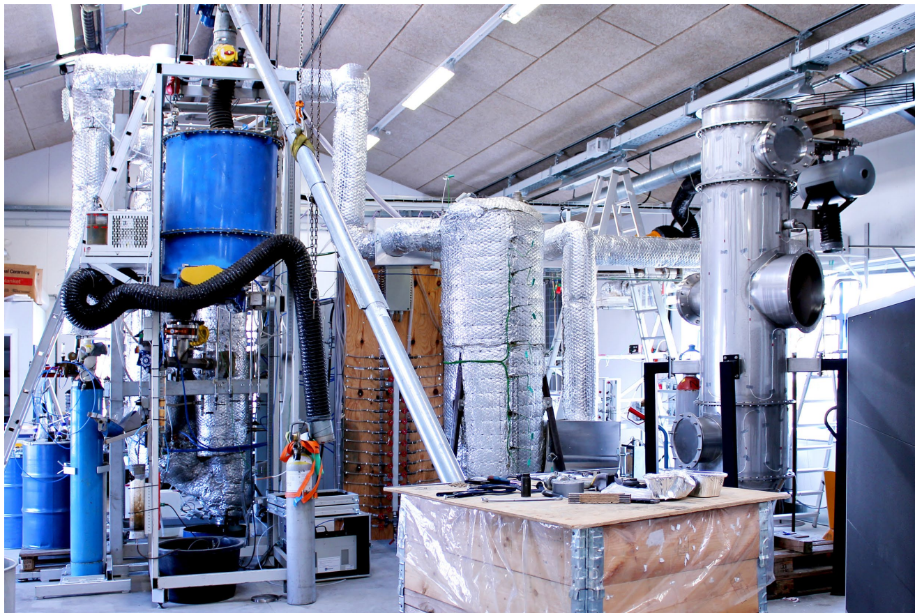
Figure 37: Picture of the only LT-CFB unit (100 kW at DTU KT, Risø Campus) currently existing. Picture taken in 2012 during installation of the ceramic candle filter (to the right). By the author.
