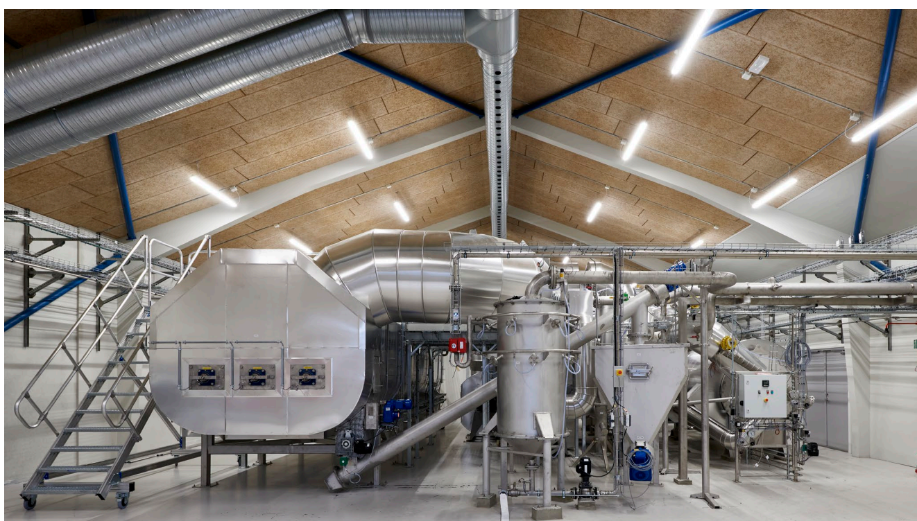
Figure 33: Picture of AquaGreen HECLA plant for steam drying and pyrolysis of sewage sludge in Fårevejle, Denmark. Picture is taken during construction. Today the plant is in full operation. © AquaGreen
