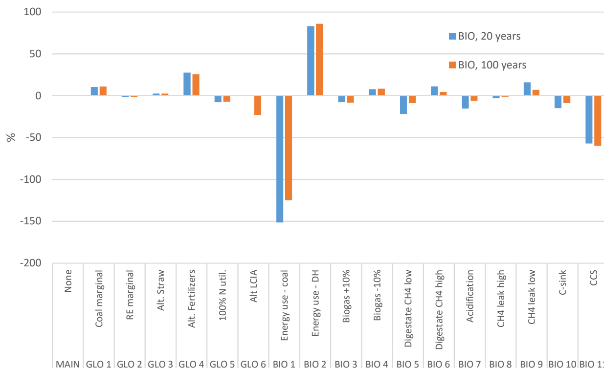
Figure 27: Relative difference of the bioogas scenario under influence of all tested parameters and compared to the main model results. A positive result implies an increased Climate Footprint of the system compared to the main model results. GLO 6 is only applicable in a 100 year perspective.
