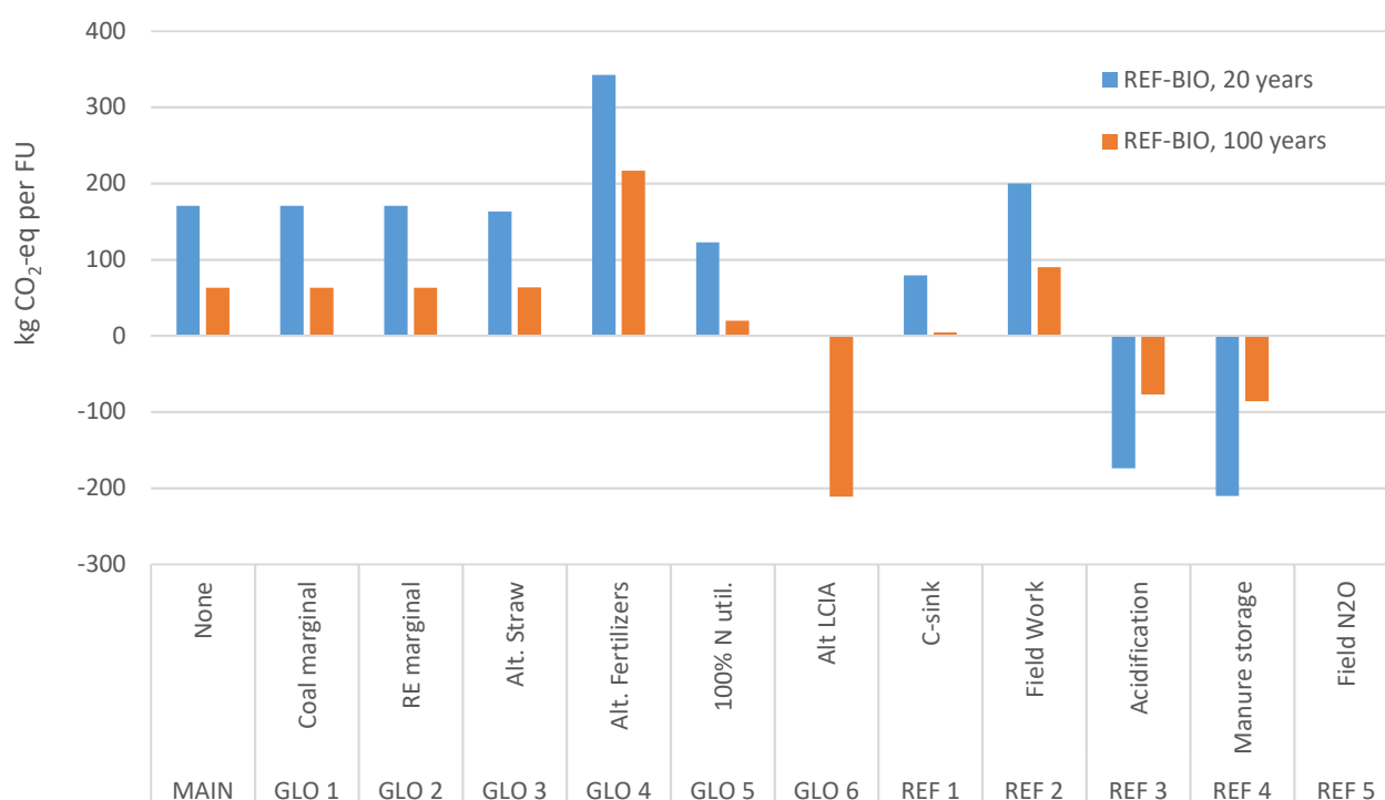
Figure 22: Absolute results of reference system for the biogas scenario with influence of all tested parameters. REF 5 is not relevant for the reference for the biogas scenario, and GLO 6 is only applicable in a 100 year perspective.
