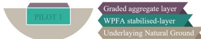
Figure 2: Distribution of layers in demonstrator service road
