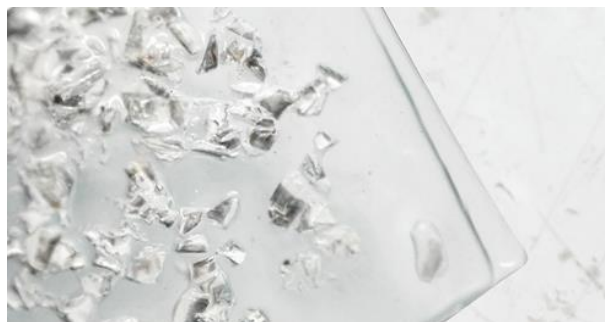
Figure 10. Fused glass plates with fish scales in between.
