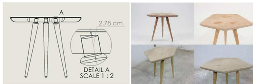
Figure 3. Detail of the second prototype and tests with different legs design attachment system to the stool base.
