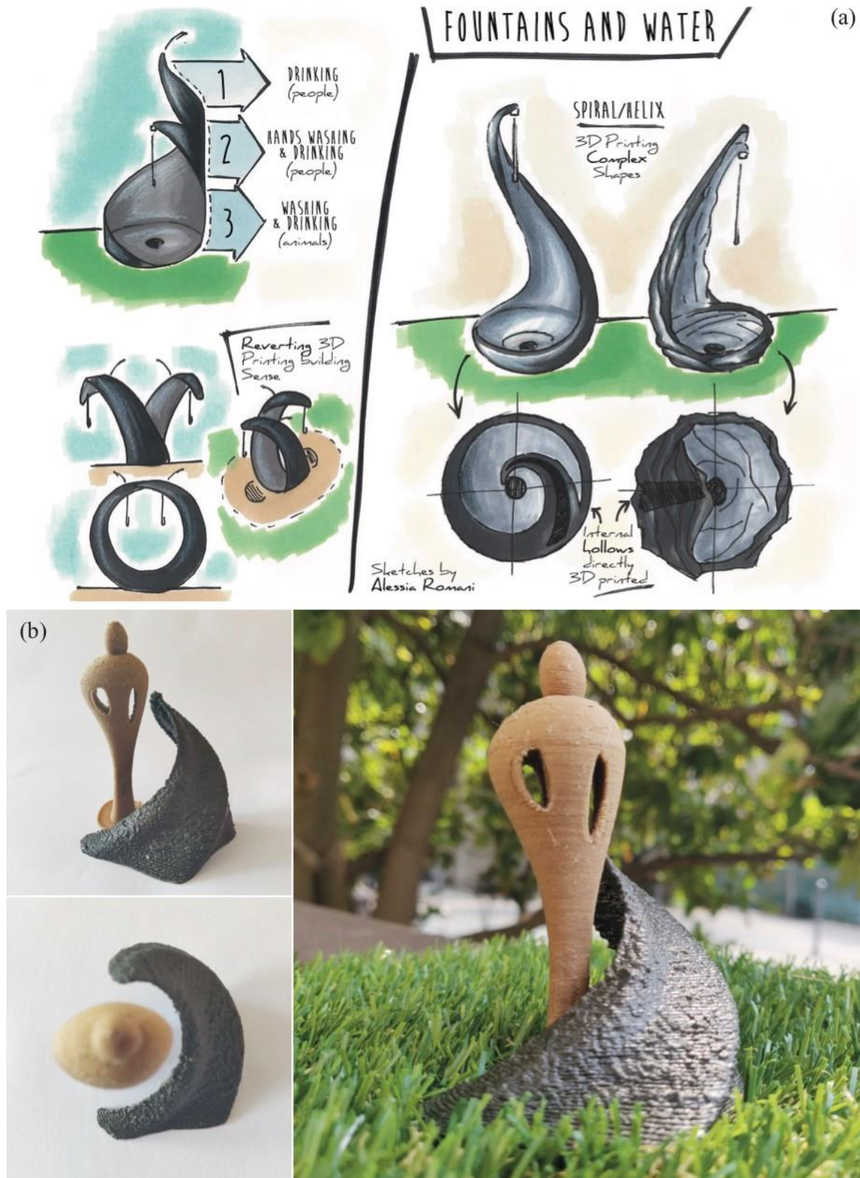
Figure 11. Additive Re-Manufacturing: (a) Design concepts of water decoration structures for urban design and amusement parks (fountains), and (b) 3D printed 1:20 scale structure obtained by LDM process with OD55R material formulation.
