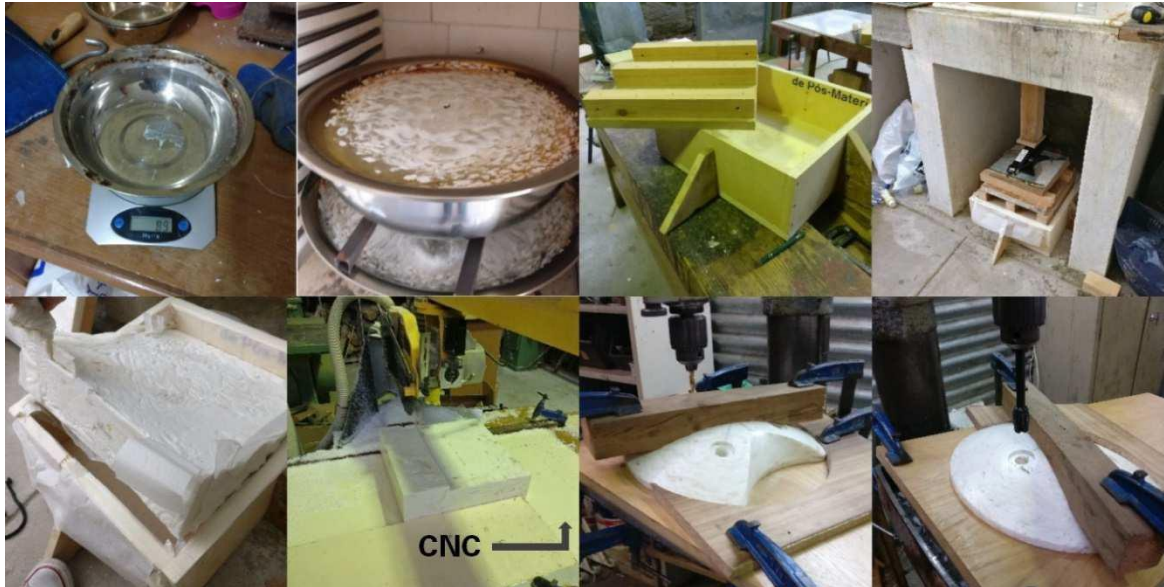
Figure 4. Manufacturing stages (from left to right); (a) weighing the plastic, (b) melted plastic inside metallic containers, (c) wooden rectangular mould, (d) application of a load during cooling, (e) retrieval of piece after cooling down, (f) rectifying into uniform rectangular shape, (g) after CNC process, making pre-holes, (h) threading holes for legs.
