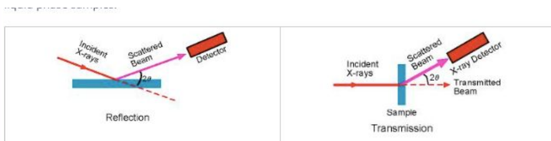
Figure 12. Reflection and transmission geometry in XRD 42 .
