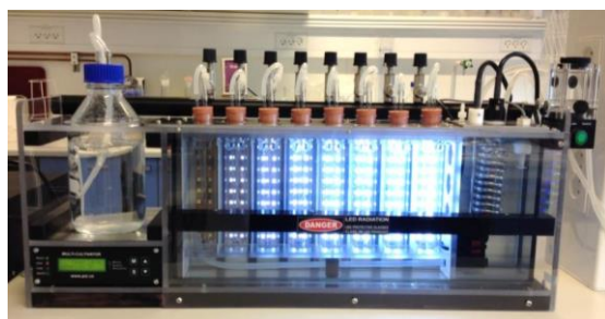
Figure 7. The table-sized PBR (Multi-Cultivator MC1000) used for the majority of the small-scale experiments with Rhodomonas . The temperature in the water-filled chamber with the culture vessels (8x 100 ml) is adjustable, and the light behind each culture vessel can be individually programmed. (Photo: C. Thoisen)
