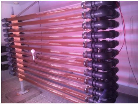
Figure 8. The tubular PBR (250 L) during a meso-scale experiment with Rhodomonas salina . (Photo: C. Thoisen)
