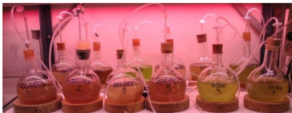
Figure 6. 1 L balloon flasks used for cultivation for some of the small-scale experiments with Rhodomonas salina . The flasks are equipped with tubes for filtered aeration (0.2 µm).
