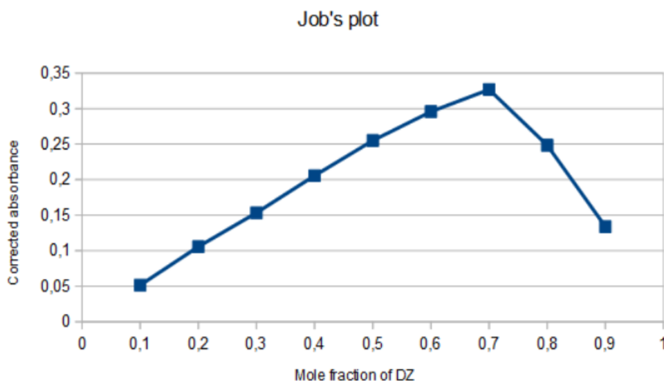
Figure 4.10: Job's plot of dithizone and mercury ion complex
