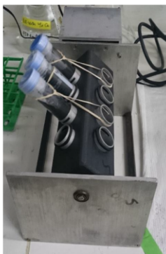
Figure S3: Rotating device developed internally at USGS used to mix spiked sediment.
