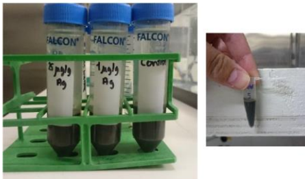
Figure S4: Exposure tubes with contaminated sediment (left) and centrifuge-tube with clean sediment for elimination (right)
