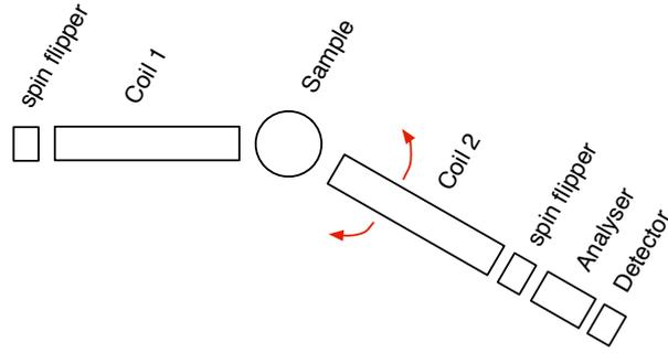
**Figure 3.8:** Schematic drawing of a typical neutron spin echo experiment. The neutron enters from the right and goes through the components. The right hand side of the sample can be rotated to cover different scattering angles.
