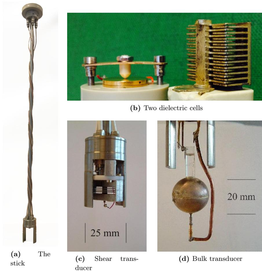
**Figure D.1:** To control the temperature during the experiments we mount a sample holder (b)-(d) onto a stick (a) and put the stick into a cryostat. We have several different sample cells and sticks, which makes for different thermal environments.
