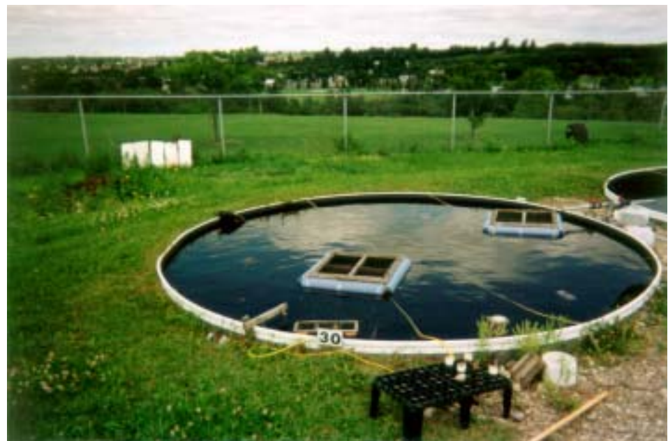
Picture 2: 12m 3 out-door PVC pond
