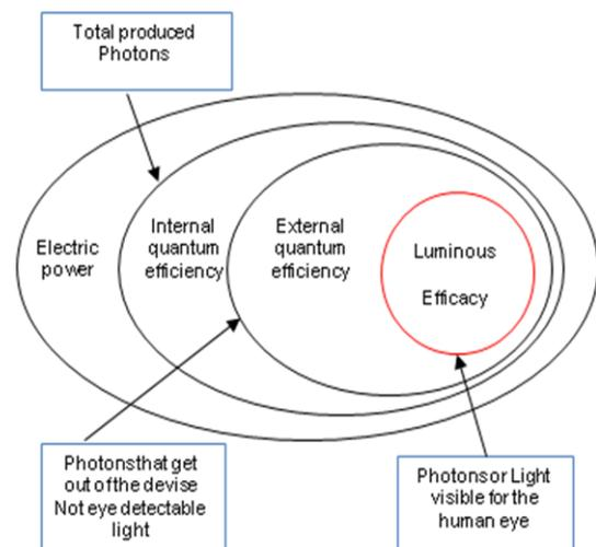
**Figure 1:** Different types of efficiency for illuminating devices.
