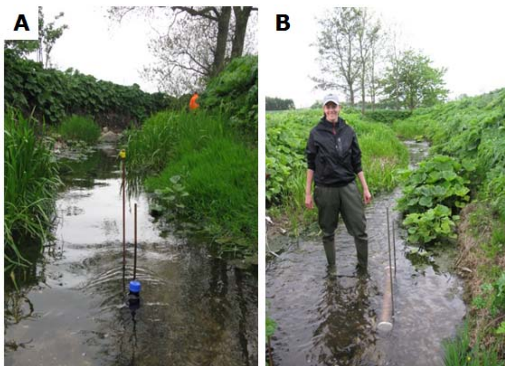
Figure 2: Photos from the field sampling in Skensved stream for the (a) event-controlled (storm-flow) runoff sampling system and (b) streambed sediment sampler.
