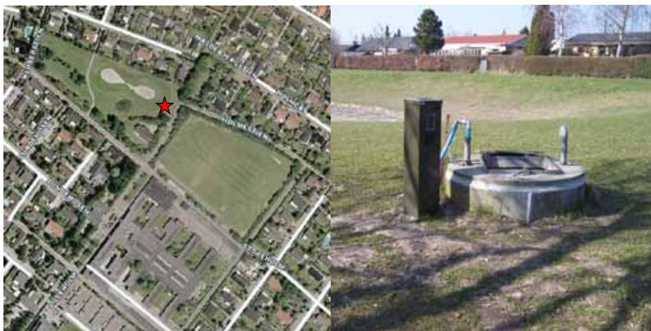
Figure 5. Location and picture of the Greve monitoring well (shown on the left by the red star). The sensors and data logger were kept inside of the concrete casing with a metal lid, shown right, which could be locked for security purposes.
