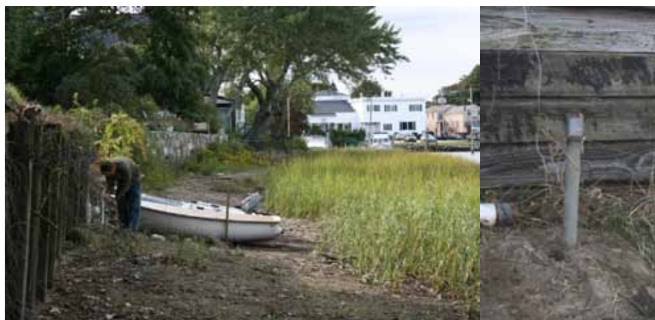
Figure 10. Pictures of the monitoring well and beach front. The left picture shows the beach front profile, with the monitoring well directly beneath the person. The right picture shows a close-up of the well with the clear thin tubing seen extending down from the bulk head and into the well.
