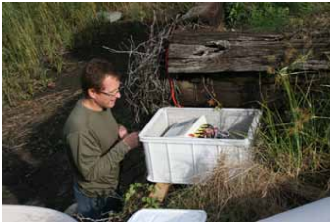
Figure 12. The container holding the sensors, pump and data-logger (on top). The container was located on top of the bulk head, just above and approximately 2m to the north of the monitoring well.
