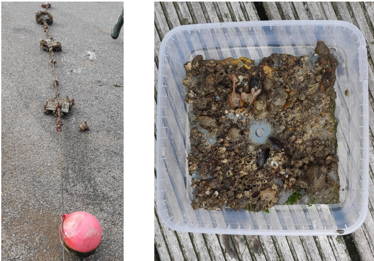
Figure 3: Left: Three settlement plates attached to a rope, which were launched in Esbjerg harbor for over 3 months. A brick is attached at the bottom end and a buoy on the top end of the rope. Right: Close-up of one settlement plate from Esbjerg harbor, which were stored in a box with ethanol after removing from the harbor until further analyses.
