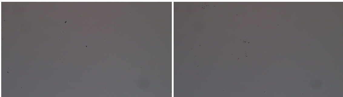
Figure 3.2: Images of a wafer which has not been plasma cleaned. There is some noticeable dust or other artefacts on the surface. Images are 10X magnified.
