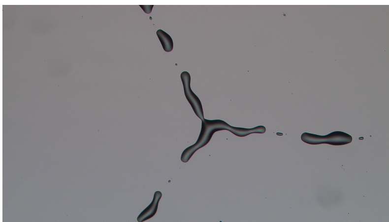
Figure 6.3: Figure showing a blob of de-wetted polymer, with strange shape. If given the mobility, the polymer would continue to break up into smaller (rounder) pieces.
