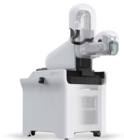
Figure 2. External appearance of Neuralink's automatic Insertion Robot for Link implantation. / Source: Neuralink Website [1]
