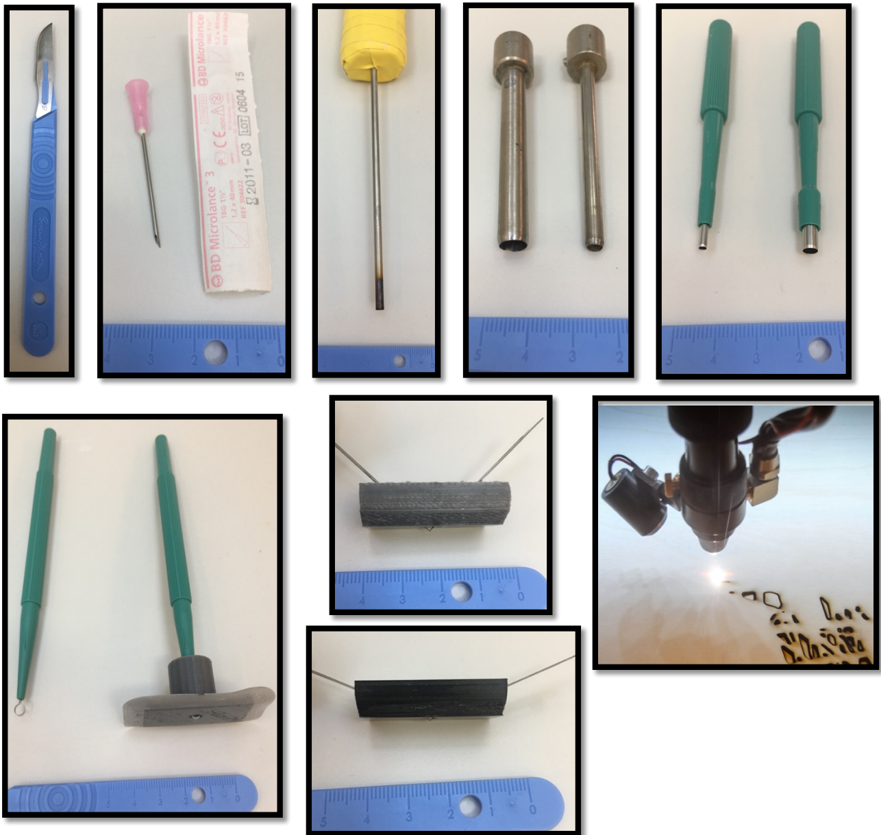
Figure 30 Pictures of different instruments tested for infliction of wounds to the porcine skin of the utilised ex-vivo wound healing model.
