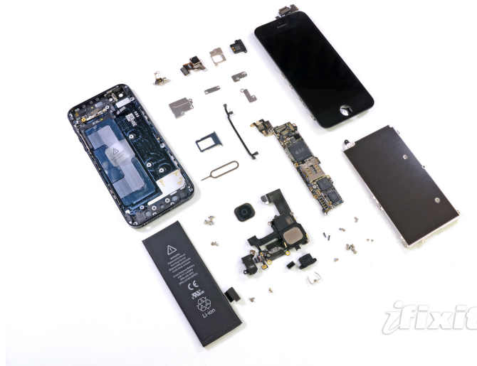
Figure 21: 'Teardown of Apple iPhone 5'. Picture reprinted, courtesy of iFixit (2013) (CC)
