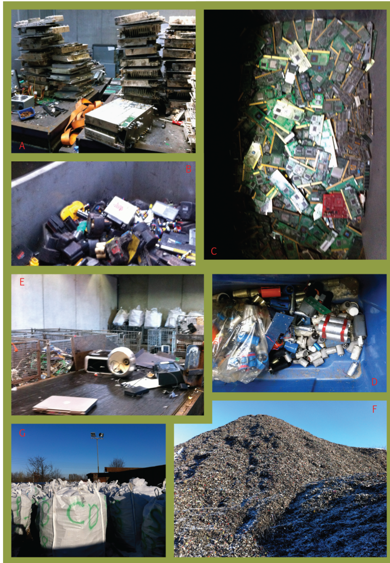
Figure 17: 'Pictures from DCR-Environment Pre-Processing Plant'. (A) Dismantling station, (B) collected mixed batteries, (C) collected PCBs from desktop computers (D) collected mixed capacitors, (E) scrap on conveyer belt, (F) granulated e-waste plastics and (G) shipping bags with different grade fractions. (Pictures by the Author)
