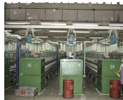
Part of the cotton dust blowing-suction system
