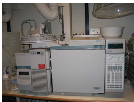
This photo is of the GC-MS in the laboratory, and shows the GC-MS from the side.
