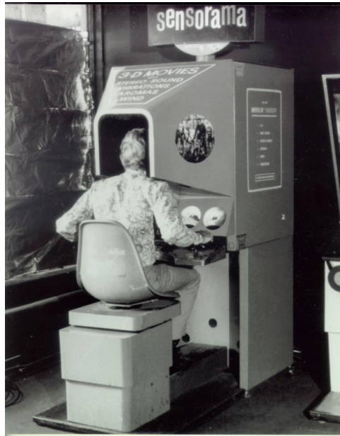
Illustration 5-3: Morton Heilig conceptualized the Sensorama in 1952 - a contraption that consists of: a stereoscopic 3D display, fans, odour emitters, stereo speakers, and a moving chair. In the Sensorama the participant could experience a bicycle ride through Brooklyn. The invention is in retrospective considered the first virtual reality technology.
