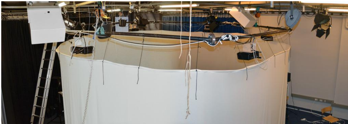
Illustration 7-3: A full view of the Experience Cylinder showing the general construction. Notice the black projectors, the rig of steel tubing, the attachment to the ceiling by the three orange pulleys, and the white canvas and its shape.
