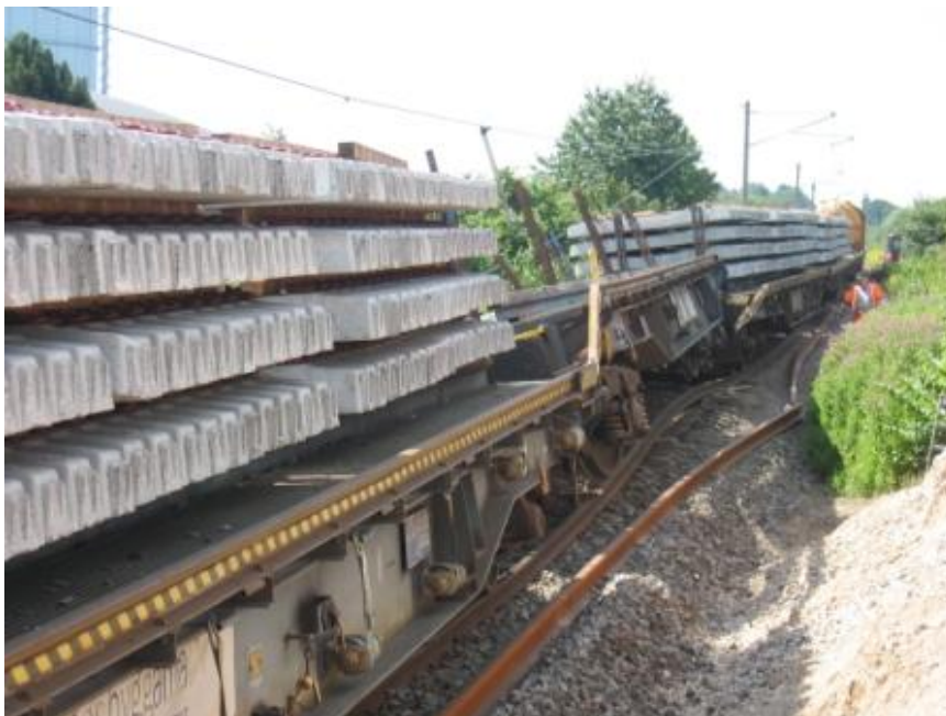
Figure 7.8: Picture of a train that ran off the railway line because of the heat on the track.
