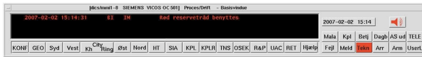
Figure 6.5: The control interface that is used as the task bar for all applications running on the user interface.
