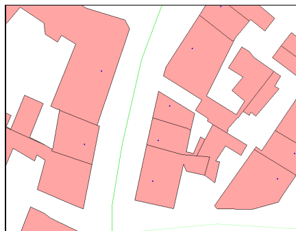
Figure 4.8 Slivers (marked dark) are formed in the process of intersecting the property theme and the buildings (left). Most slivers are removed by an automatic approach supplemented by manual removal (right).
