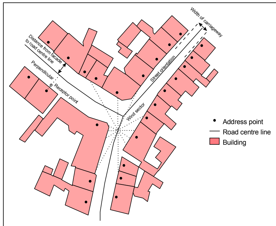
Figure 4.16 Street configuration parameters generated by the urban landscape model for use in the OSPM model to calculate air pollution levels. The digital map includes building polygons, address points, and polylines to represent the road centre lines.
