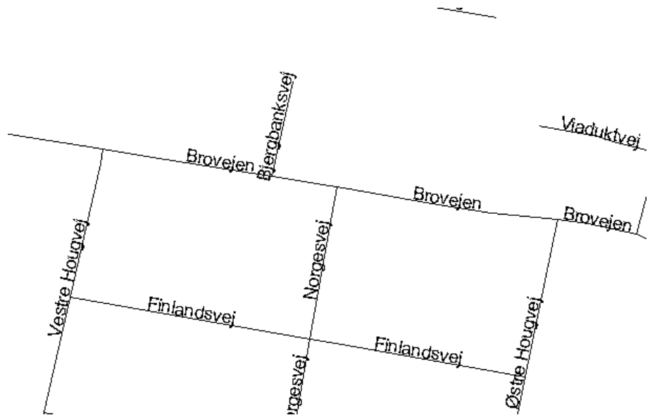
Figure 4.13 The geocoded road network with street names. A street may extend over several street intersections.
