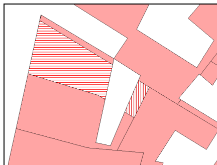
Figure 4.7 The intersect procedure may form a composite polygon (multipolygon) that is composed of two polygons (left). These composite polygons are identified and simplified into two separate polygons (right).
