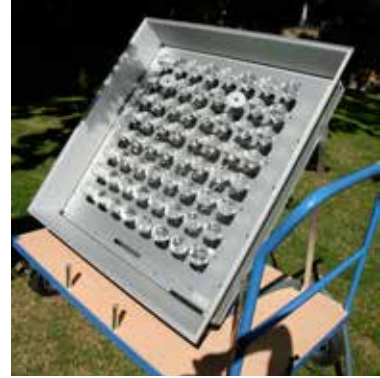
Picture 4.5: (right) Solar optical fiber collector system
