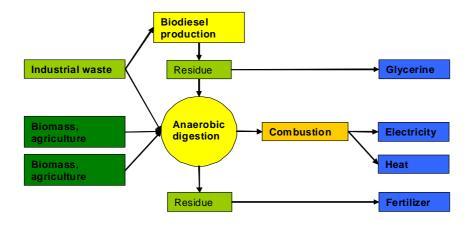
The system illustrated above combines two biofuel production lines. One that converts slaughterhouse waste (fat) into biodiesel and a second one which use the slaughterhouse waste directly in the biogas reactor. The two systems can also be combined in a system in which the residue (glycerine) from the biodiesel is utilised in the biogas plant. The use of the residue from the biodiesel production will be determined by the market price for glycerine as glycerine is also used in competing products.
