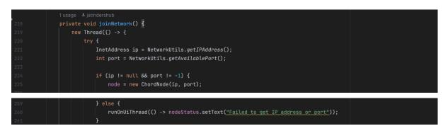
The *joinNetwork* method handles the logic for a node joining the network. It is executed in a separate thread to avoid blocking the UI thread. This can be seen on line 219.
