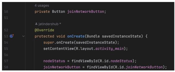
The *joinNetworkButton* variable gets declared of type Button on line 50. The variable then finds the button view in the UI using its ID *joinNetworkButton* through the *findViewById* class on line 58 and assigns it to the declared variable.
