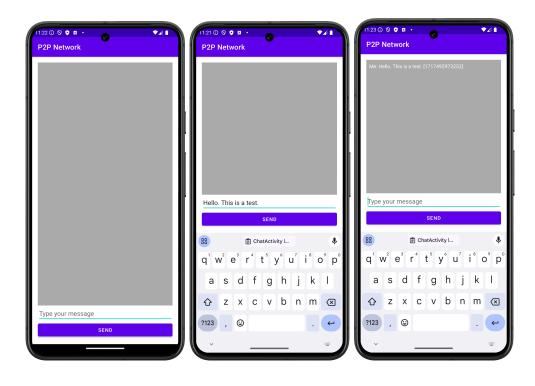
When launching the *activity\_chat.xml* the user is met with a large area intended to display the chat messages, an input field with the placeholder "Type your message", and finally an "Send" button (see the left picture above for visual context).
