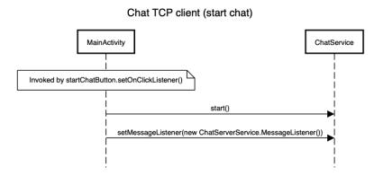
*MainActivity* sets up a button click listener to extract the IP and port, create and start a *ChatService* instance, and log incoming messages via a listener. *ChatService* connects to the server, sets up communication streams, starts *ChatActivity*, and listens for messages in a separate thread, forwarding them to the listener.
