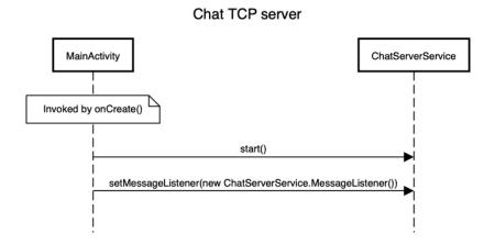
The startServer method in MainActivity initializes the server setup by creating a new thread that calls the method startServer in the ChatServerServices. The *ChatServerService* then initializes a *ServerSocket* to listen for incoming client connections on a specified port. When a client connects, it accepts the connection and spawns a new thread to handle the client's communication, allowing the server to manage multiple clients concurrently.
